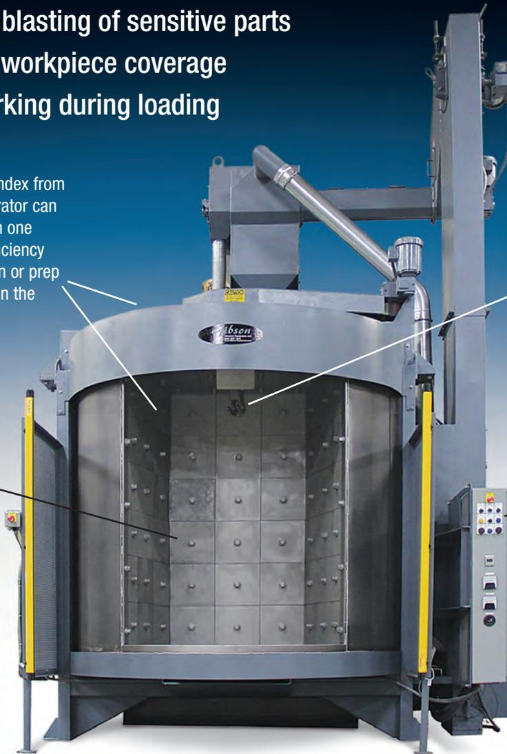
Gibson Spinner Hangers provide an ideal solution for batch blasting many types of parts too fragile or awkward for other methods of automated finishing. These systems play a profit-boosting role across a broad range of metal-intensive industries by improving quality and efficiency during the cleaning, peening, prepping and finishing of almost any workpiece suitable for mounting on hooks.
