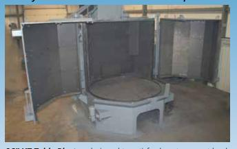
**96" XT Table Blaster**, designed to satisfy almost any part loading requirement, processes workpieces weighing up to 10,000 pounds with diameters to 96 inches and heights to 84 inches.
