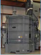
**84"** Table Blaster, with a part capacity of up to 10,000 pounds, includes a V-notched top for center loading with a crane.
